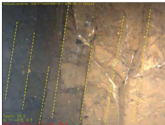
Figure 8.1.1: Depth 36.5m (front camera). Near-vertical stratification as seen in the south wall of the shaft. Small cross veins of calcite with millimetre to centimetre in size are seen. These veins are crossing the stratifications with an acute angle, the most important on the right side of the picture.
