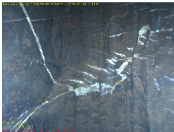
Figure 8.1.33 Calcite veinlets occupying en echelon tension joints showing syntectonic mineralisation. Winding shaft 37m.
