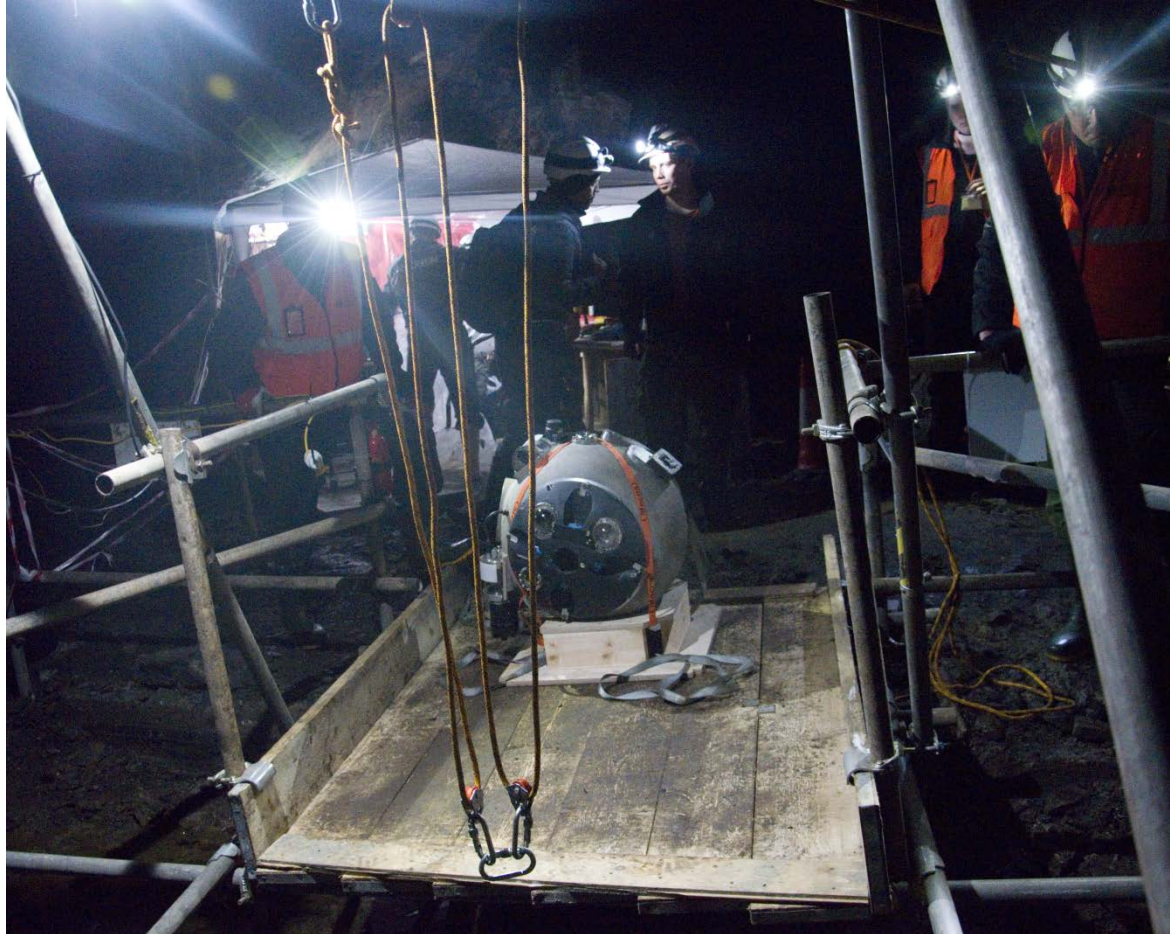
Fig. 7.15: The dive platform at the pumping shaft, photographed just after a submersible arrived for the first time (Photograph: John Barnatt).
