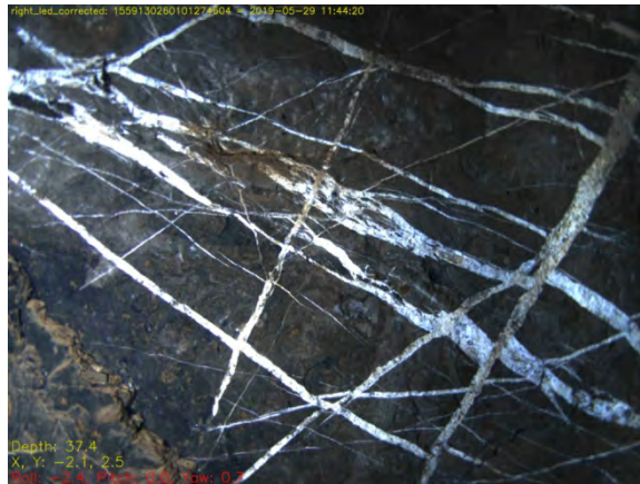
Figure 8.1.31 Multi-phase calcite veining with movement on fracture planes. White LED illumination. Winding shaft, -37m.
