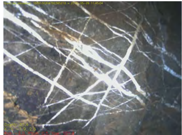
Figure 9.33: ?three phases of cross cutting calcite veins in hydraulic fractures. Note displacement of earlier veins by later ones (-37.4m Winding Shaft).
