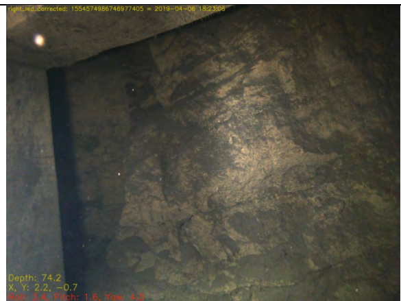
Figure 3.6 Evidence that fine sediment is lying on the less vertical surfaces and giving a false impression of colour contrasts in the granite
