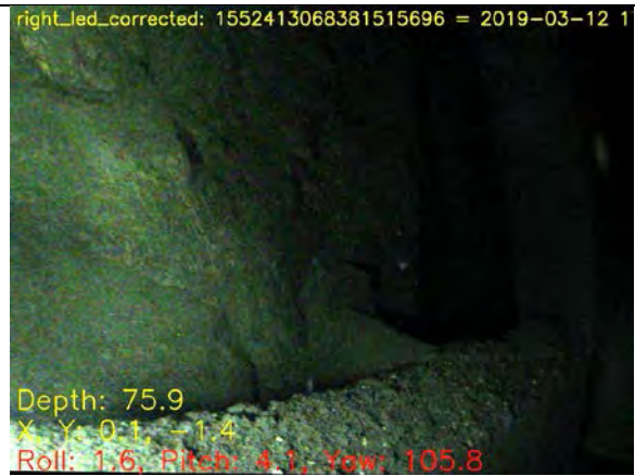
Figure 3.4 Yellow staining on broken surface of granite. Unfortunately there are no ultraviolet-source images or multispectral data for this part of the mine to assist identification.
