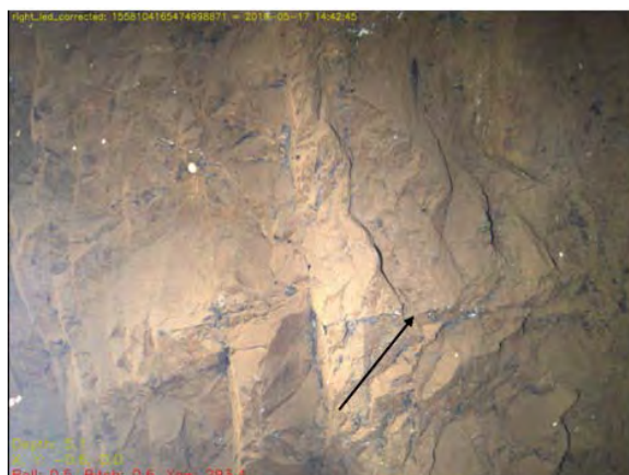
Figure 8.1.35: Depth 5.1 (Right camera). A system of fractures, mostly horizontal, filled with a black mineral (alteration?)
