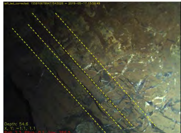
Figure 8.1.4: Depth 54.6m (left camera). Thick bedded limestone with apparent dip to W about 50°
