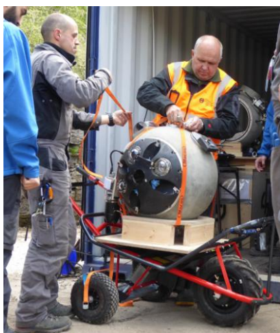
UX-1A robot in its cradle on the electric trolley for transfer into Ecton Mine
